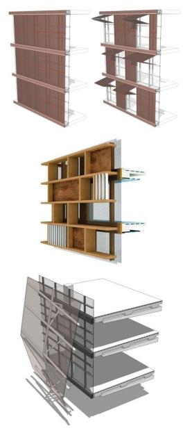
Fig. 5. 3D computer models of envelope assemblies
